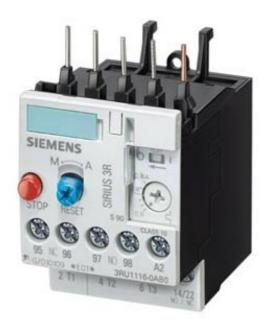
OVERLOAD RELAY 0.45...0.63 A FOR MOTOR PROTECTION SIZE S00, CLASS 10 FOR CONTACTOR MOUNTING MAIN CIRCUIT: SCREW CONN. AUX. CIRCUIT: SCREW CONN. MANUAL-AUTOMATIC-RESET
