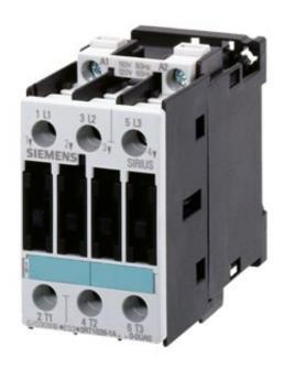
CONTACTOR, AC-3, 11KW/400V, AC 110V 50HZ/120V 60HZ, 3-POLE, SIZE S0, SCREW TERMINAL
